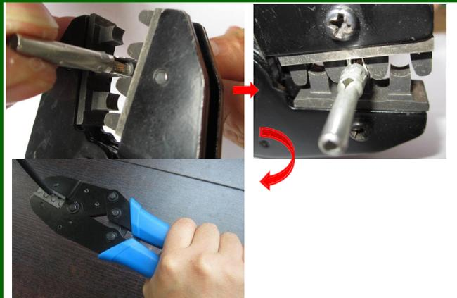
Step 6: riveting is completed.
