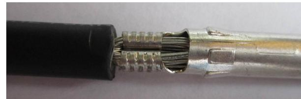
Step 7: assemble the connector.
