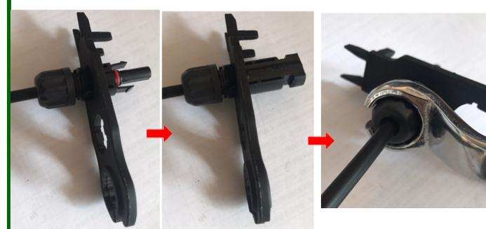
Step 10: adjust the clearance of the nut to 0.2 - 0.8 mm.
