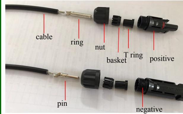
Step 4 : cut the cable before installing the connector (strip 9mm).
